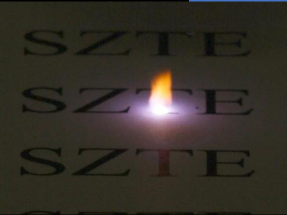
Plasma formed on a text by the infrared pulse of a Nd:YAG laser (wavelength 1064 nm)
