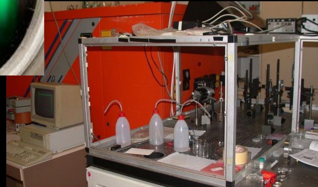
Ultraviolet pulses from KrF excimer laser (wavelength 248 nm) can easily form plasma in vacuum. Target: copper
