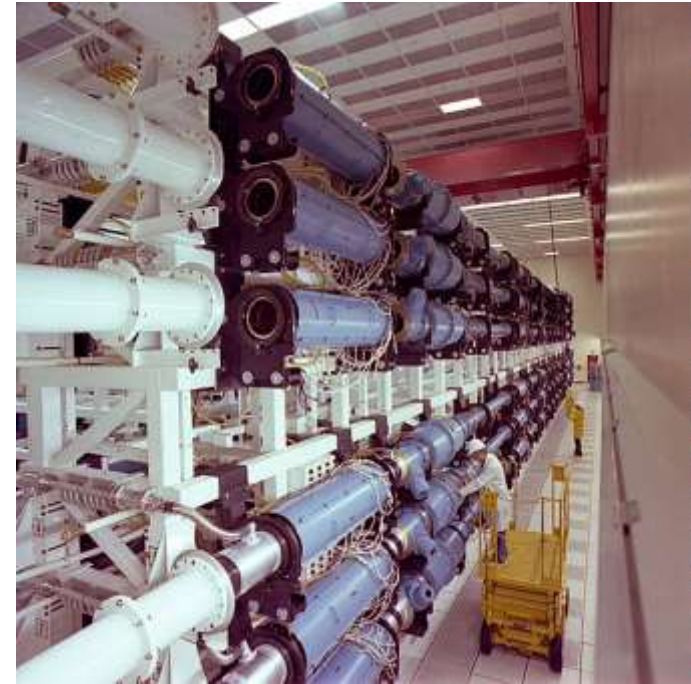
Amplifier chain of the SHIVA laser at LLNL, late 1970's (Nd:Glass 10 kJ, 1 ns)
